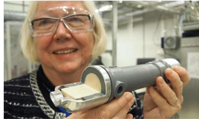
May Britt Hägg, a professor in the Department of Chemical Engineering at the Norwegian University of Science and Technology holds the CO 2 membrane separator she and her research group have developed. Credit: Per Henning, NTNU
