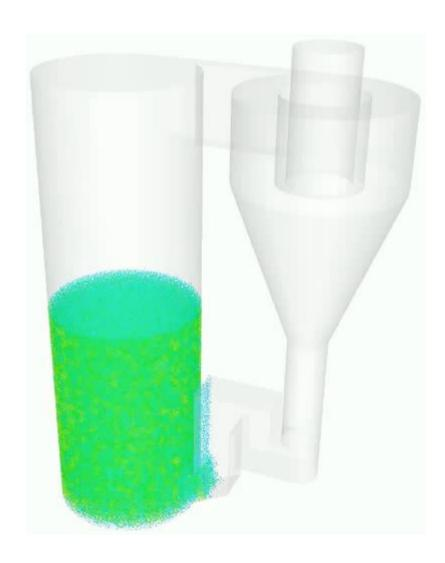
Simulation of 12 m circulating fluidized bed with cyclone and loop seal
