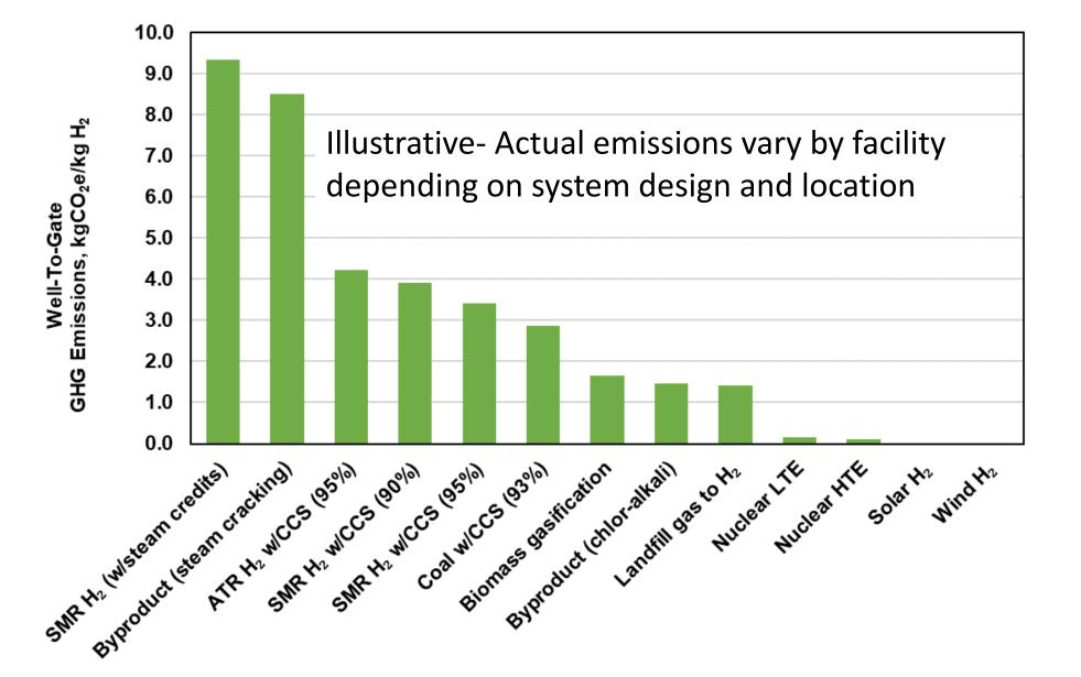
SMR= Steam Methane Reforming; ATR=Autothermal Reforming CCS=Carbon Capture and Sequestration; LTE=Low-Temp Electrolysis; HTE=High-Temp Electrolysis; LFG=Landfill Gas
