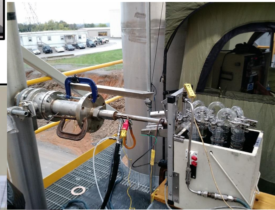
Manual Emission Sampling for Amines, NH 3 , Aldehydes, Nitrosamines
