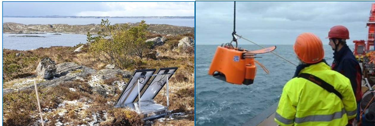
Coastal and offshore deployments of Broadband seismometers
